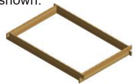
16. Once you have reached the desired working platform height. Correctly fit your Toe-board system as shown.
