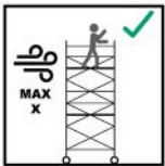
Do not build, dismantle or attempt to work on an access tower if the wind speed exceeds 17MPH
