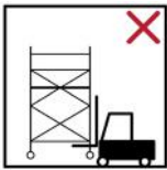
Do not lift the tower with mechanical equipment
