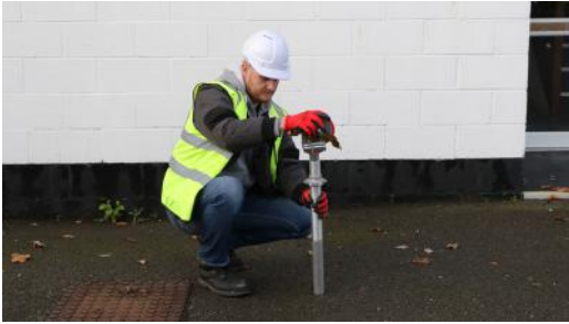
1. Insert castor wheels into adjustable legs
