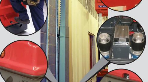
Repositioned charger - for extra protection to water ingress when power washing
