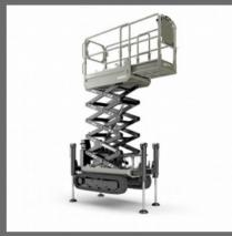
BIBI, mini-crawler scissor lift able to operate at 8 m working height. The crawler traction overcomes all the standard limits of traditional 4x4 traction providing the opportunity to work in limited spaces. The automatic levelling of the machine, enables the operator to work easily and always in full safety conditions even in big slopes or uneven and rough terrain. The bi-energetic engine, thermic and electric, provides full versatility, both for inside or outside applications.
